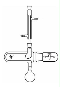
08-1000: DRYING APPARATUS, ABDERHALDEN - For use in vacuum/vapor type drying operations. Consists of one West type condenser, one jacketed drying chamber with ■ 34/45 joint, one desiccant tube with ■ 34/45 joint and vacuum connection with one solvent flask.
