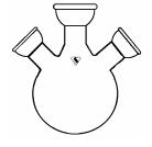
05-1380HW: FLASK, ROUND BOTTOM, THREE-NECK, HEAVY WALL - Same as 05-1360 except side necks are at a  $20^\circ$  angle.
