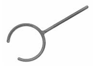
05-3080: LOWER SUPPORT RING FOR REACTION VESSEL – Support ring is constructed of  $\frac{1}{2}$ " OD epoxy coated stainless steel rod. Made with an opening for easy insertion of reactor with an 8" long rod for connection to lattice.
