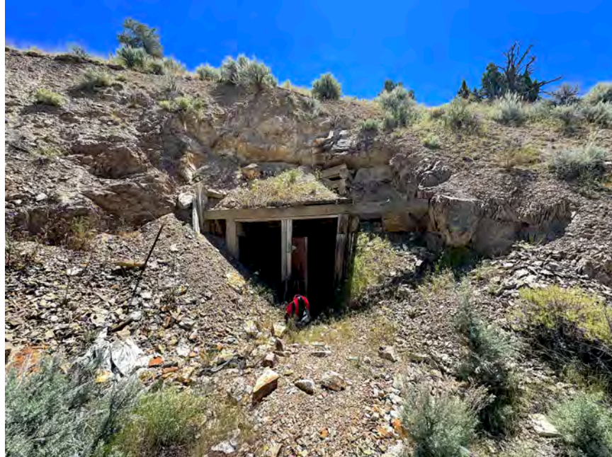
Figure 11: Looking south at the No Name adit; note the latite dyke
