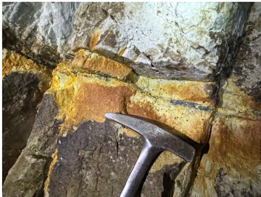
Figure 25: Close up of antimony mineralization in fractured, altered latite, lower Arrance adit, with yellow antimony oxides (cervantite?) bleeding out of the fractures, lower Arrance workings
