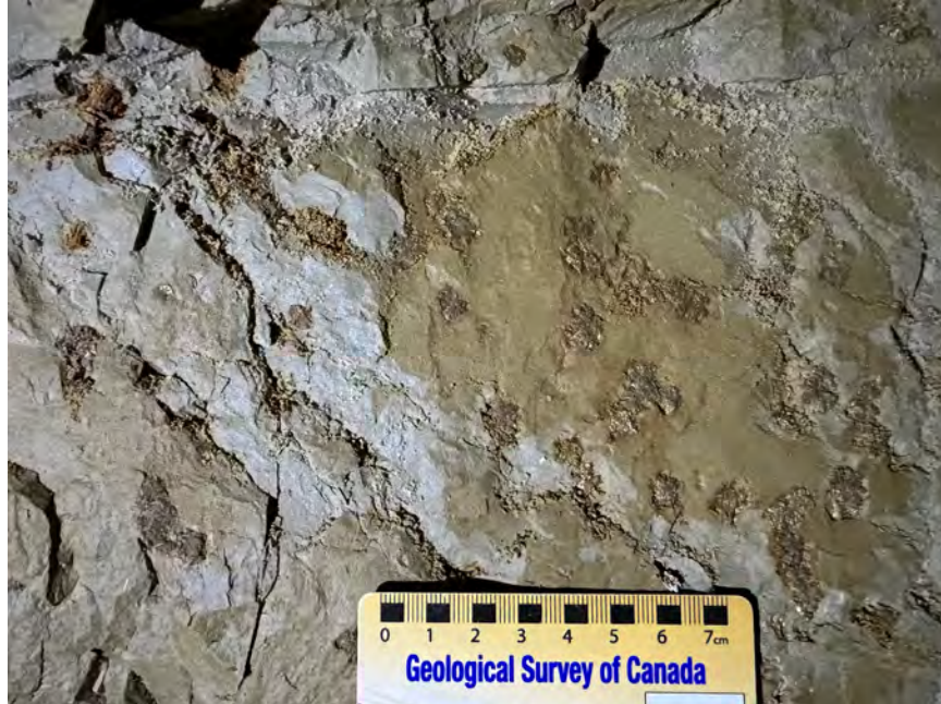
Figure 26: Subhedral “clots” of pyrite in otherwise unmineralized, moderately silicified limestone, lower Arrance workings
