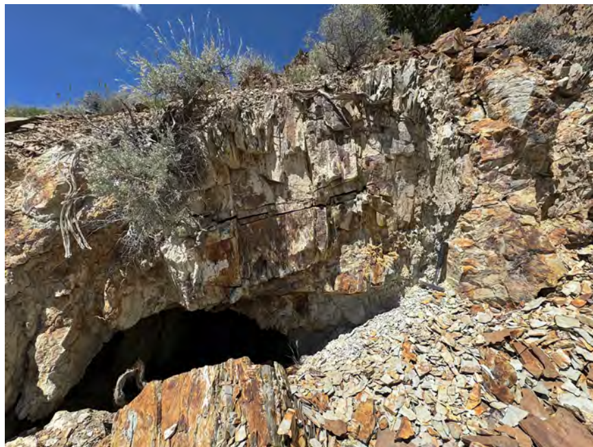
Figure 35: Inaccessible adit, middle Hoyt workings, in roughly north-south, wide, steeply-dipping, deformed, slaty sandy shale
