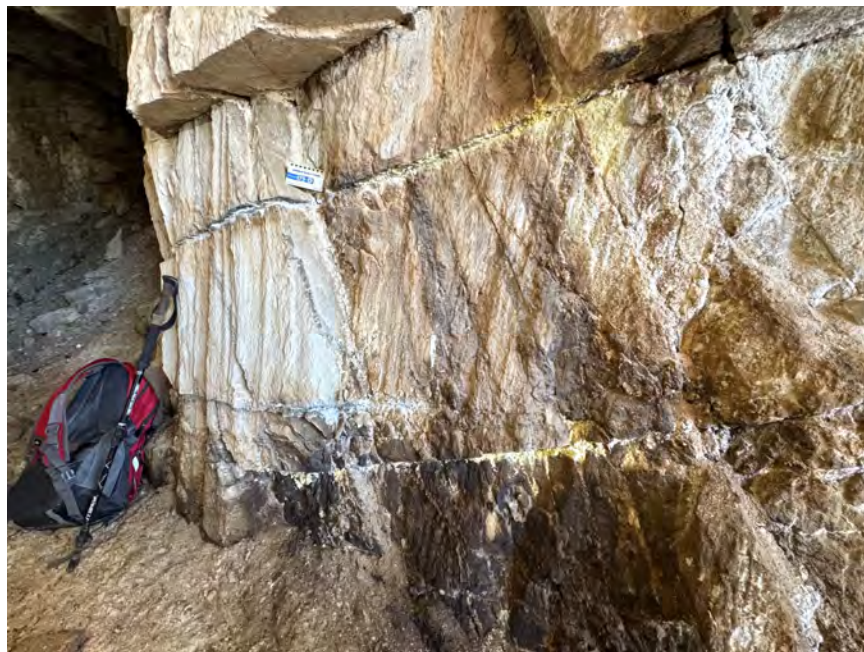
Figure 21: Mineralized orthogonal fracture set in the wall of the middle Arrance adit, in banded and/or sheared contact of the latite dyke
