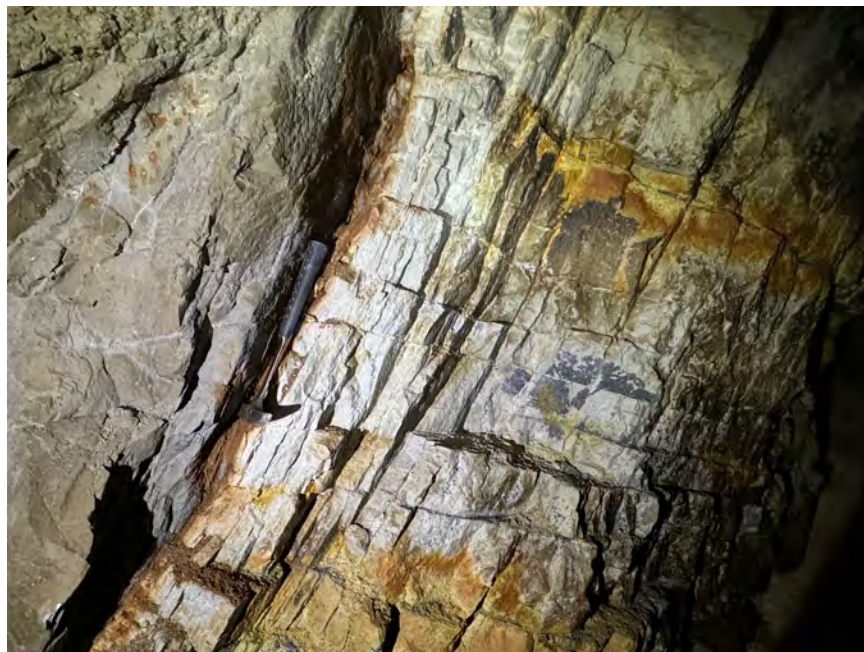
Figure 23: Further along the adit, steeply west-dipping hanging wall contact of the fracture-controlled mineralized altered latite dyke and weakly pyritic limestone, lower Arrance workings
