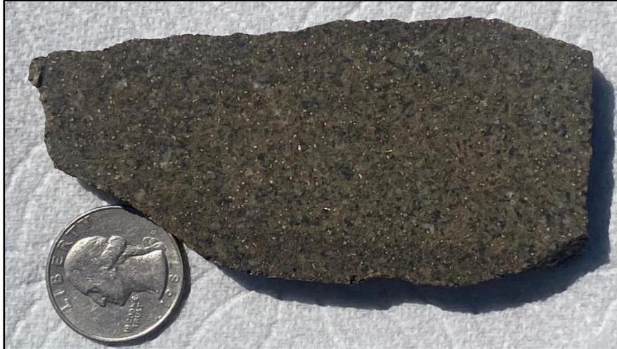
**Figure 4. Photo of medium-grained, equigranular monzonite occurring as sills and dikes emplaced into the Triassic siltstone within Bernice Canyon.**
