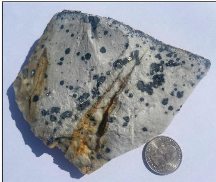
**Figure 12. Fine-grained, QSP altered felsite with disseminated pyrite enveloped by stibnite spheres and clots, Arrance mine dump. Sample #969121 contained 2.45% Sb.**
