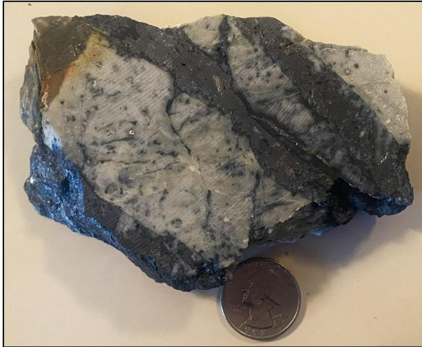
**Figure 13. Photo of massive stibnite veins cutting QSP-altered felsite; minor stibnite stringers and clots present in the felsite, Antimony King mine (see Figure 5).**
