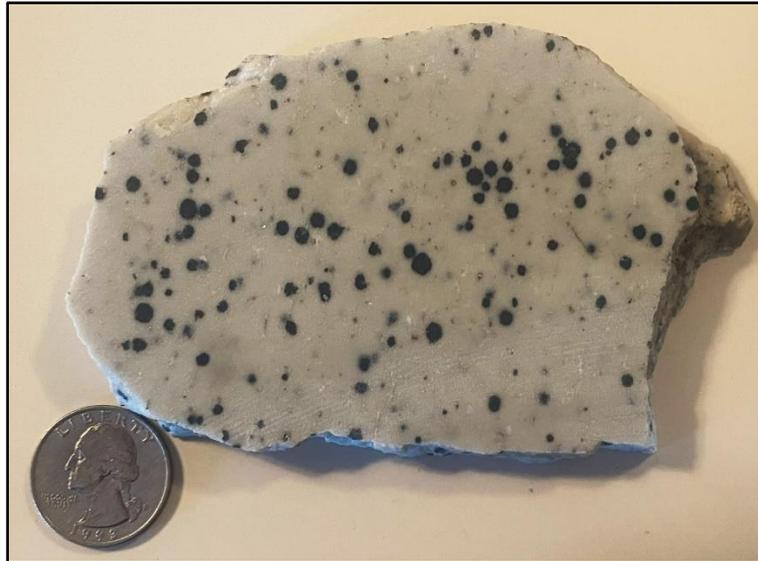
**Figure 11. Photo of disseminated, stibnite-rich spheres in strongly QSP altered felsite, Arrance mine dump. Sample #969113 contained 1.69% Sb.**
