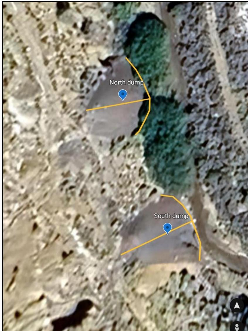
**Figure 22. Aerial view of the Antimony King mine area and the two dumps estimated in the volumetric study.**
