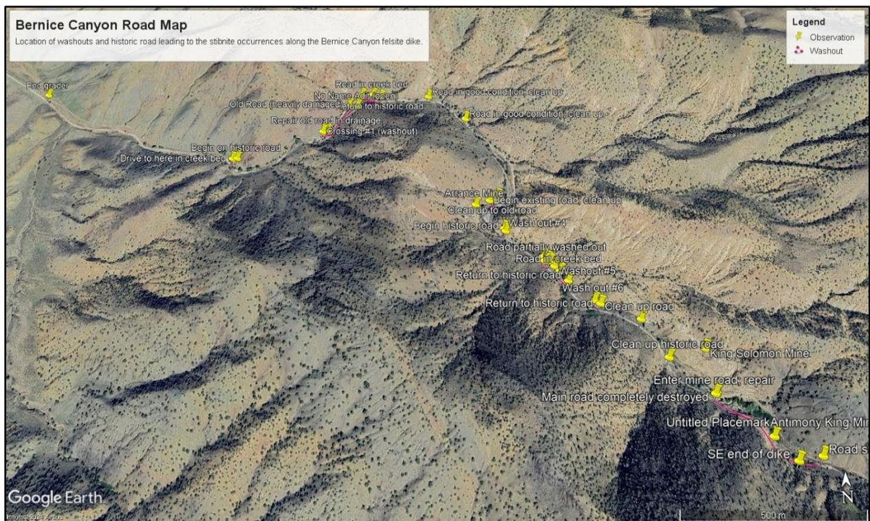
**Figure 21. Aerial view of Bernice Canyon showing the trace of the historic road into the antimony mines. Washouts (#1 - #6) are show in red and the description of the proposed work to rehabilitate the road is provided in Table 2.**
