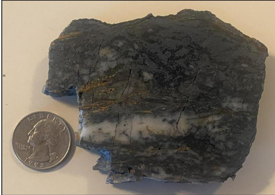
**Figure 14. Photo of vein-like stibnite occurrence developed along the sheared felsite-siltstone contact; gray = massive stibnite, black = carbonaceous, sheared rock; white = milky quartz; orange = iron oxides/ankerite veinlets, Antimony King mine (see Figure 6). Sample # 969124 contained 30.89% Sb, 8.3 ppm Ag and 0.24% Zn.**
