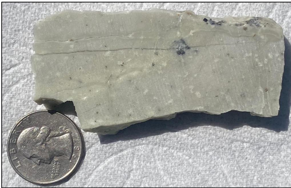
**Figure 9. Photo of the pervasively sericitized felsite with relict fine-grained, plagioclase phenocrysts and disseminated pyrite-stibnite clots. Note several crosscutting stages of quartz-sericite, quartz and quartz + sulfide micro-veinlets, King Solomon mine.**
