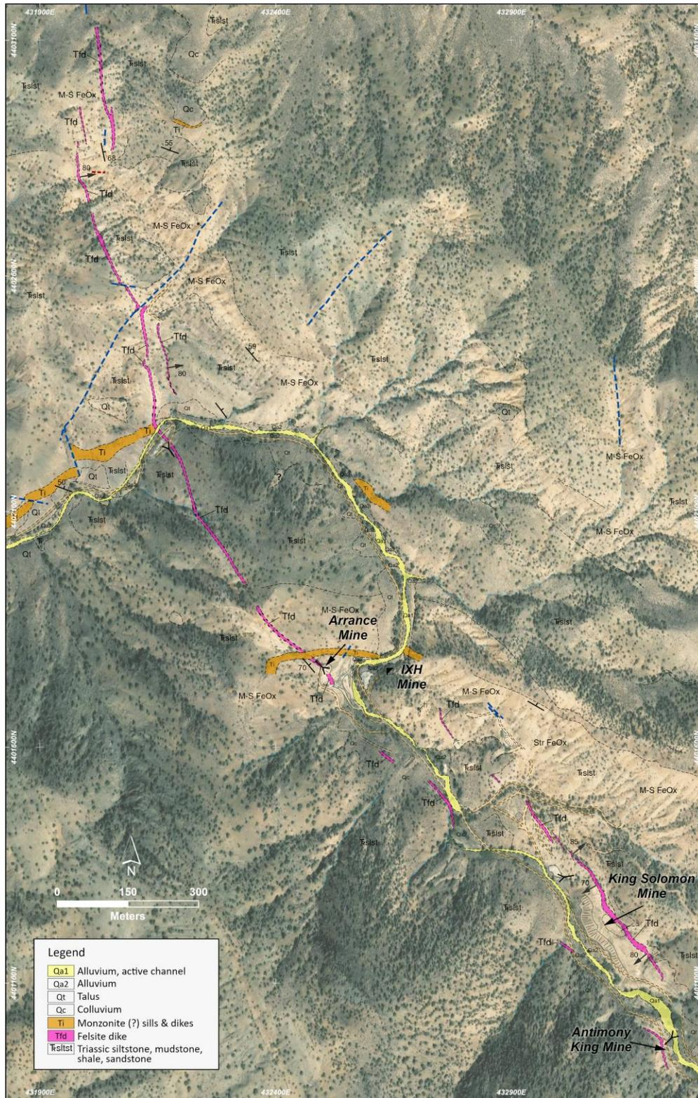
**Figure 6. Preliminary geologic map of the Bernice Canyon area showing the distribution of antimony mines and stibnite occurrences along the extent of the felsite dike complex.**
