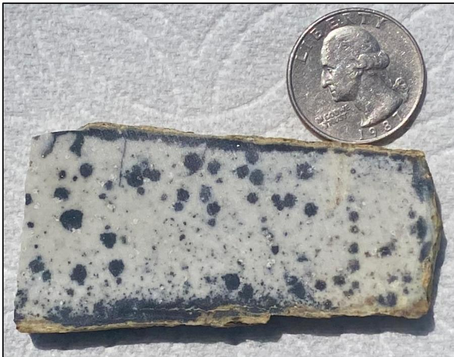
**Figure 15. Altered felsite with parallel, stibnite-rich veinlets (sub-horizontal) with stibnite 'bleeding' or replacing into the felsite, IXH dump. Sample #969114 contained 0.77% Sb.**
