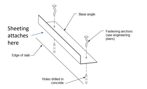
This is the formed base angle that we provide. This piece lays flat on the slab and the sheeting sits on this lip so each piece lines up exactly the same. When installed with the bottom closure strip, the sheeting is sealed.
