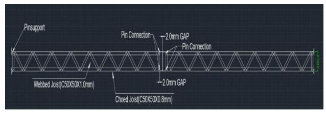
Figure 20. Common joist types (Case1)
