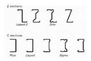
Figure 3. Cold-formed steel section type
