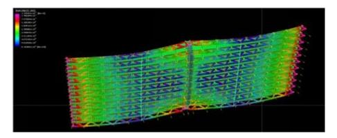
Figure 39. Colour chart for Beams displacement(Case1)
