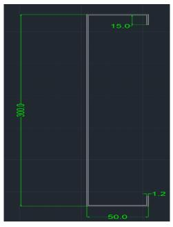
Figure 21.The "C" joist type(Case2)
