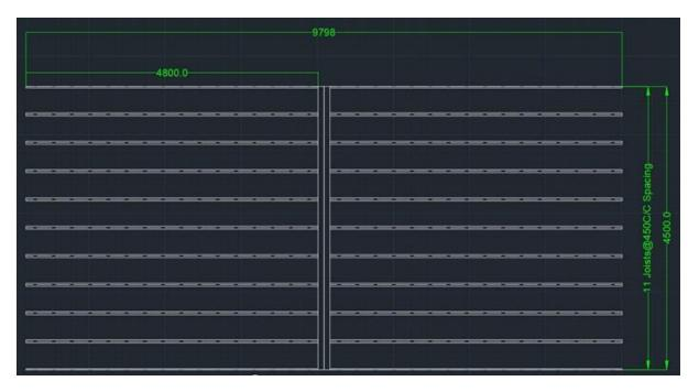
Figure 17. Dimensional drawing of the floor slab (mm)
