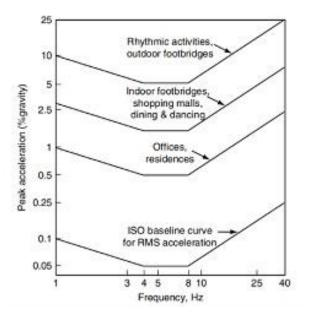
Figure 6. ISO acceleration limits (Resources from: ISO 1989)
