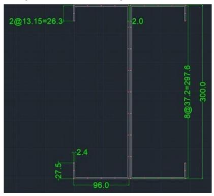
Figure 18. Beam cross section and dimensions (mm)
