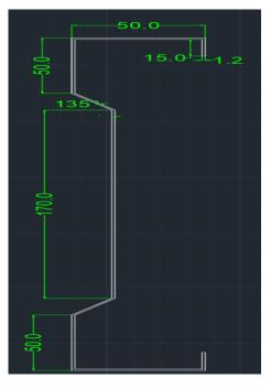
Figure 22.Cross-section of a "dumbbell" joist(Case3)
