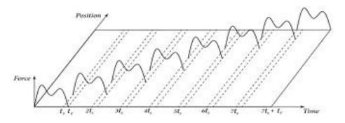
Figure 9. Loading scheme of single-footfall force (Resources from: Zhang & Xu, 2020)
