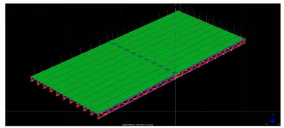
Figure 30. Axis settings for flooring systems
