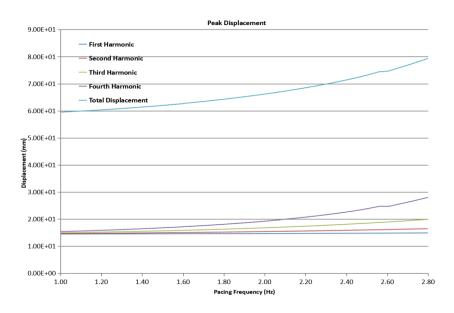
Figure 60. Peak Displacement(Case3)
