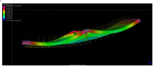
Figure 41.Colour chart for Beams displacement(Case2)
