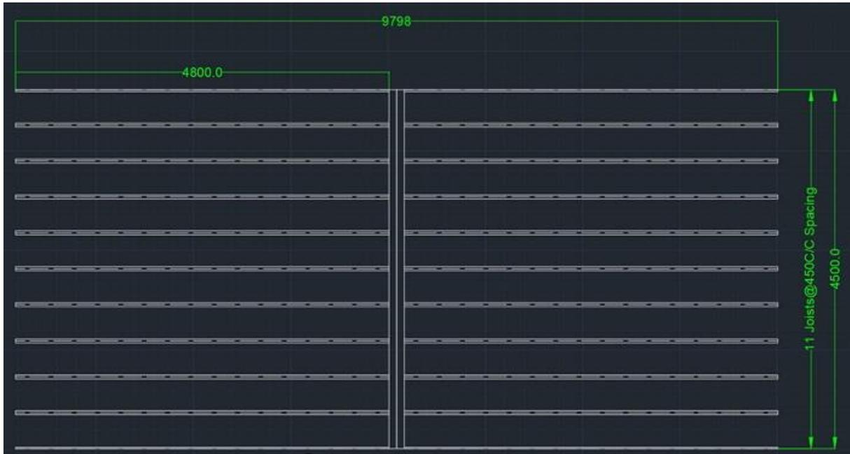
Figure 17. Dimensional drawing of the floor slab (mm)
