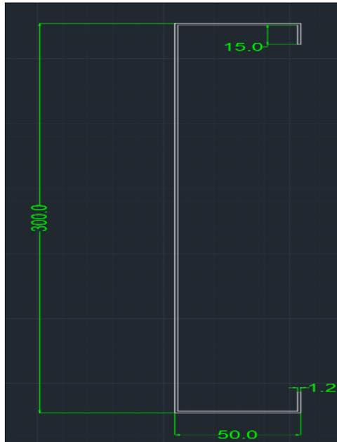
Figure 21. The "C" joist type (Case 2)
