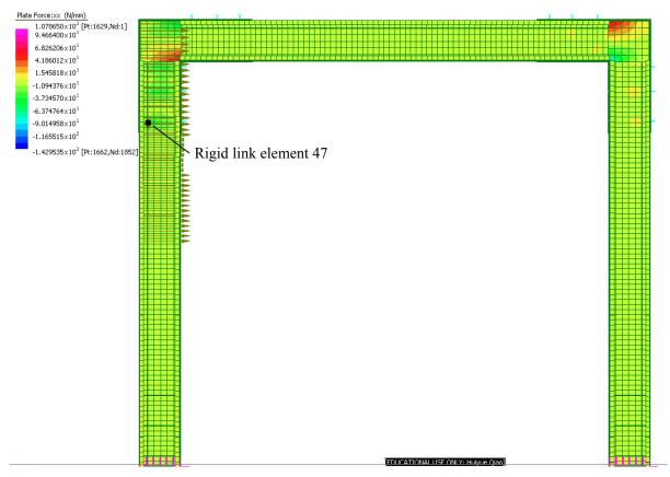
Figure 25. Plate force contour plot front view.
