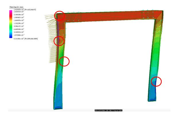
Figure 24. Deformation shape of the portal frame model at the ultimate load.
