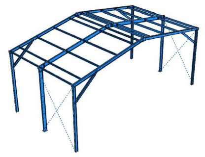
Figure 12. Finite element model for tested portal frames (Rinchen & Rasmussen, 2019)
