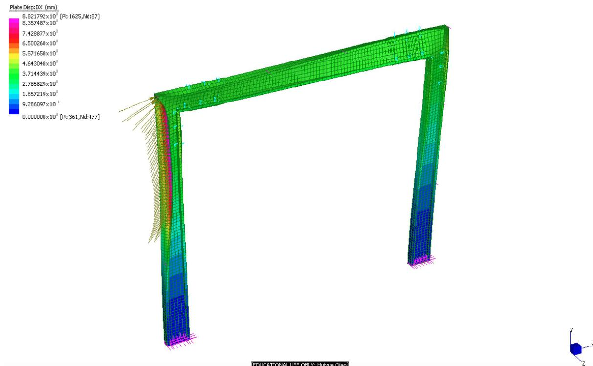
**Figure 23. Global deformation shape of the portal frame under designed wind load**
