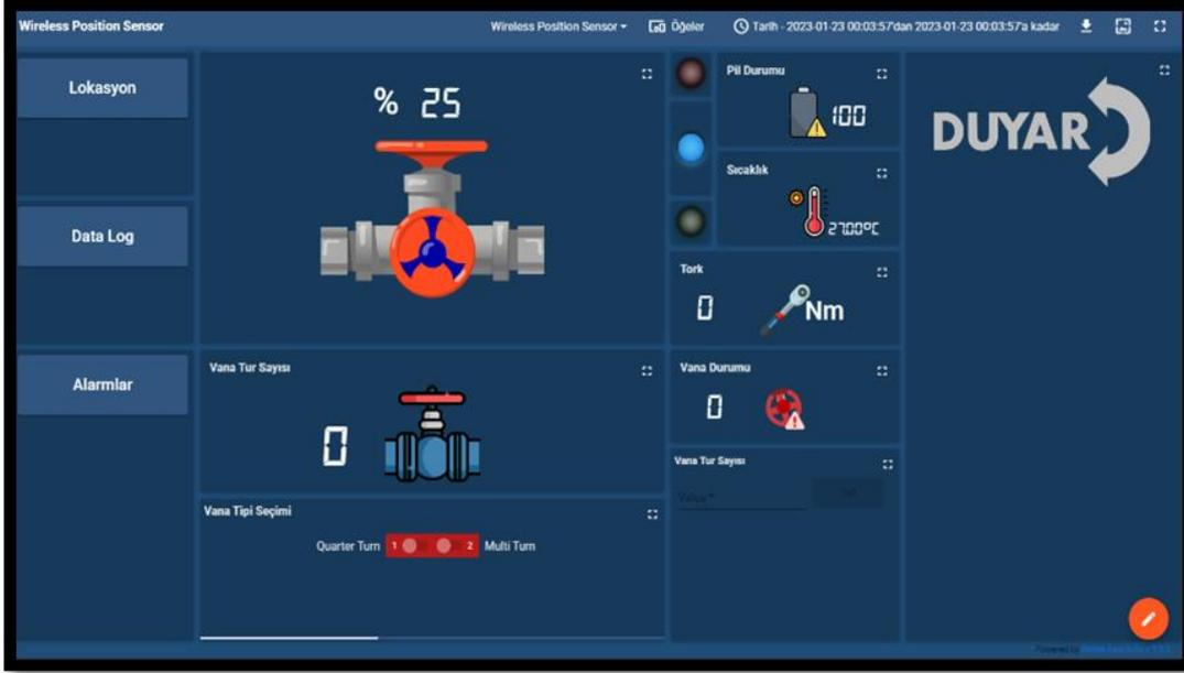
Duyar IoT Wireless Position Sensor to the hand wheel or lever of a manual valve, it is able to measure and monitor via the cloud dashboard the position of the valve (in real time, valve open- valve closed or intermediate Position) It has alert section that is able to demonstrate when the set threshold is exceeded.
