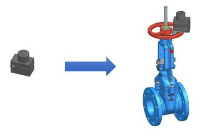
2- Adjust the valve in fully closed and turn the slider button on (it automaticly calibrate itself) .
