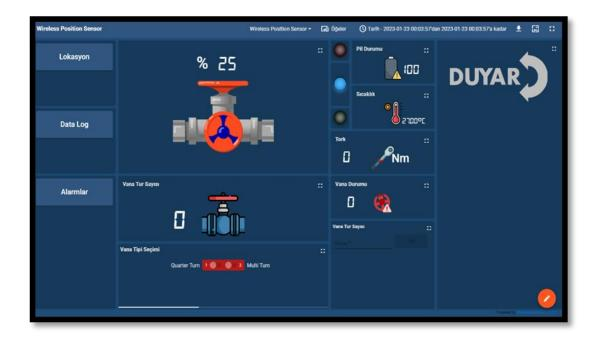
Duyar IoT Wireless Position Sensor to the hand wheel or lever of a manuel valve, it is able to measure and monitor via the cloud dashboard the position of the valve (in real time, valve open- valve closed or intermediate Position) It has alert section that is able to demonstrate when the set threshold is exceeded.
