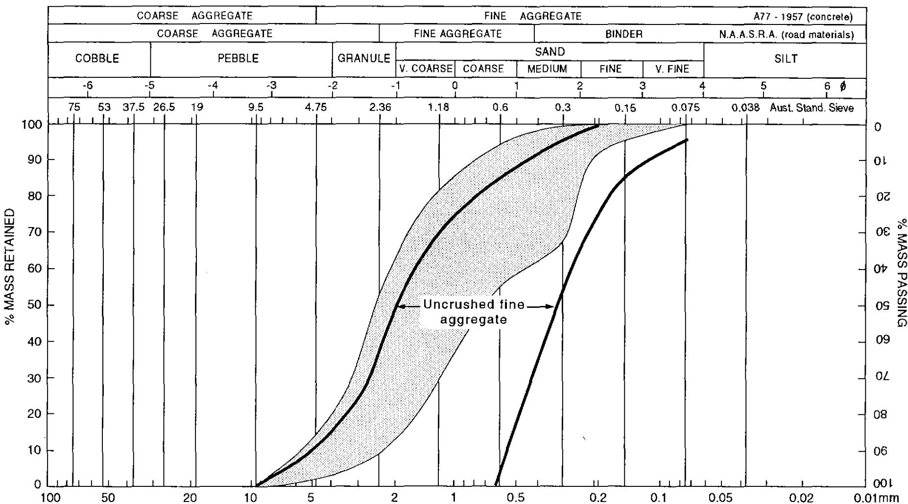
Figure 3 - Grading Envelope: Pioneer Fine Aggregate
