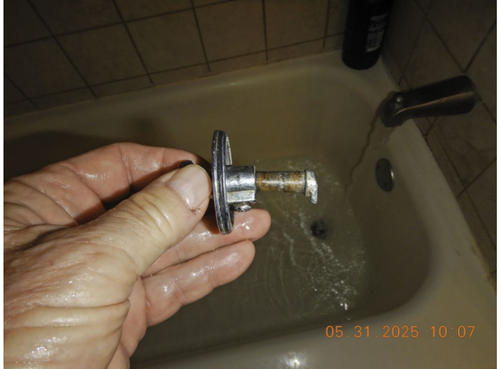
Damaged drain plug.
