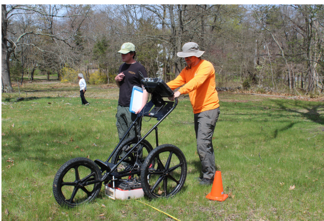
Figure 7 GPR Device operated by archaeologists Olivier Vansassenbrouck and Vaughn Ortner. Equipment like this can cost between $30,000 and $40,000. This is a major factor in the cost of doing GPR.
