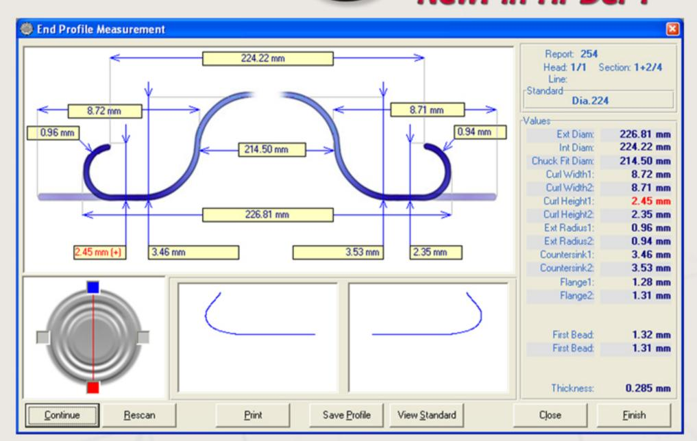
The End Profile Analyzer uses laser profiling technology to measure sanitary can ends. The system measures the following measurement values:
