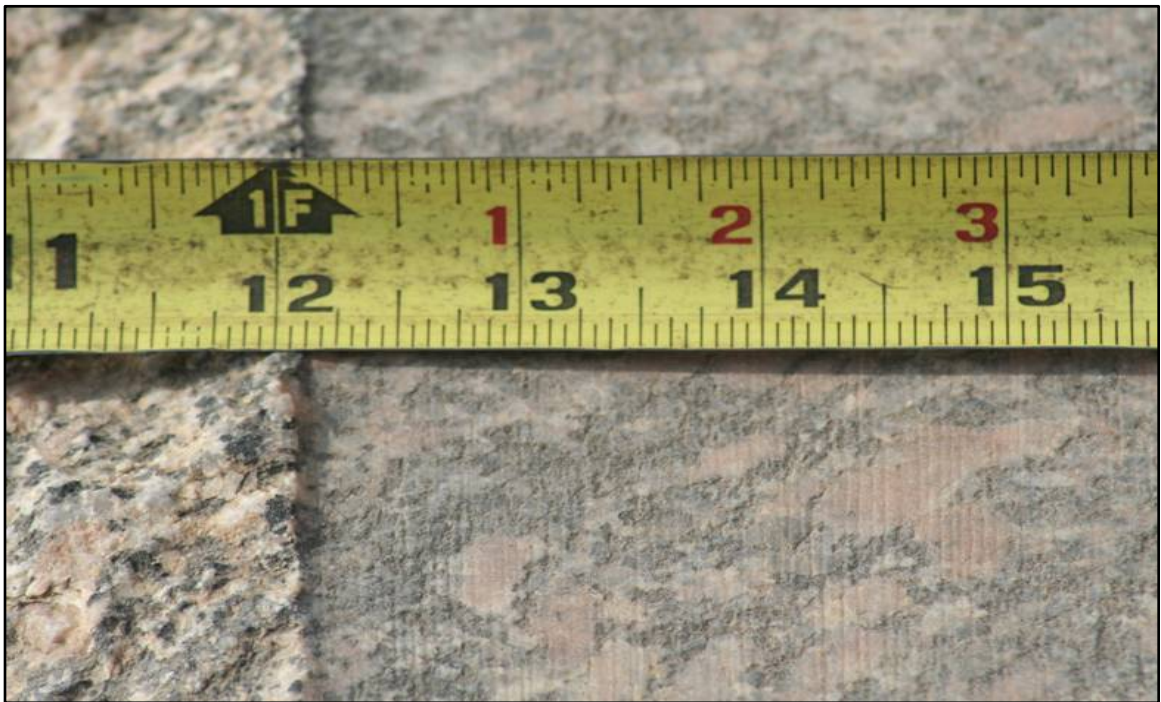
Figure 5. Clear evidence of machine feed marks
