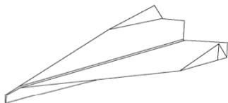
Fold the wings down along fold lines 5 and the winglets up along fold lines 6. Add wing dihedral by tilting the wings up slightly away from the fuselage. The wings will have a slight "V" shape when viewed from the front. You are ready to fly!
