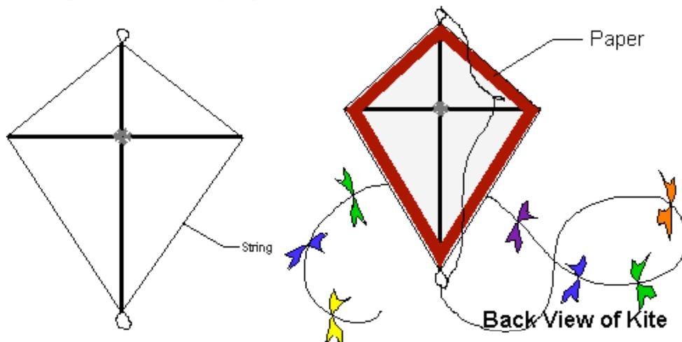
6. Make a tail by tying a small ribbon roughly every 4 inches along the length of string. Attach the tail to the loop at the bottom of the kite.
