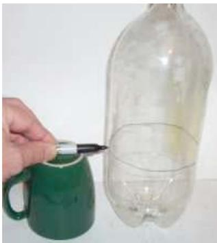
**Step 1:** Draw a line around the bottle about six inches up. You can use a neat little trick to make a nice straight line - rest the marker on the top of an upside down coffee cup then I rotate the 2 liter bottle. It makes a nice straight line.
