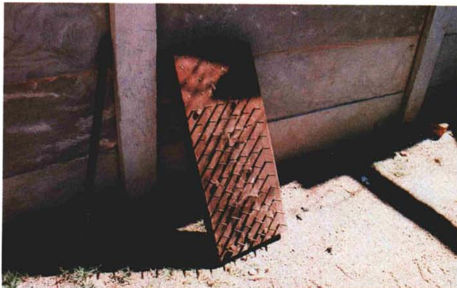
This homemade verticutter is a board with 3-inch nails pounded through it. A rope is tied to it, someone stands on it and then it's dragged across a green.
