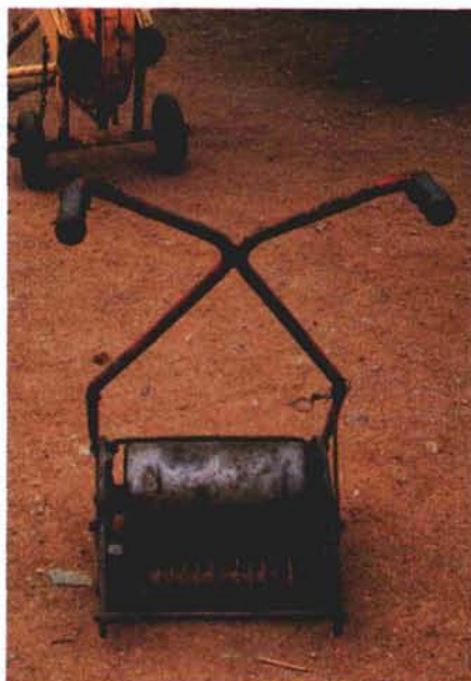
Another version of a homemade verticutter.
