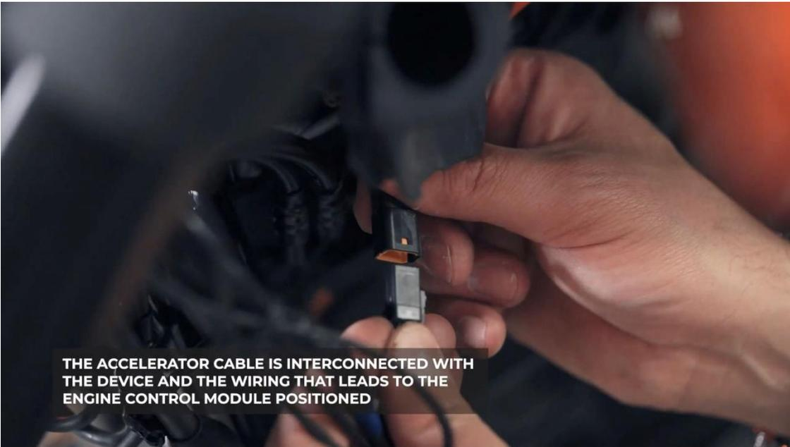
**THE ACCELERATOR CABLE IS INTERCONNECTED WITH THE DEVICE AND THE WIRING THAT LEADS TO THE ENGINE CONTROL MODULE POSITIONED**
