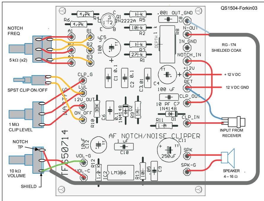
**Figure 3** — Connections between controls and the circuit board. (Bournes, CTS, NKK components from [digikey.com](http://digikey.com)).
