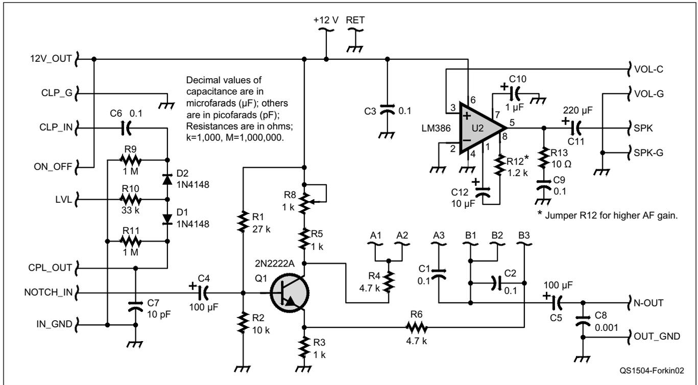
**Figure 2** — Schematic diagram of the notch filter/clipper board. (Stackpole, Yageo, Vishay BC, Panasonic components from **digkey.com**; Kemet parts from **mouser.com**).
