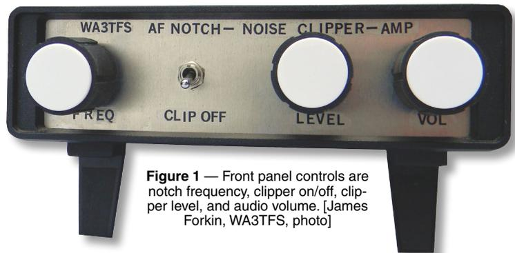
Figure 1 — Front panel controls are notch frequency, clipper on/off, clipper level, and audio volume. [James Forkin, WA3TFS, photo]
