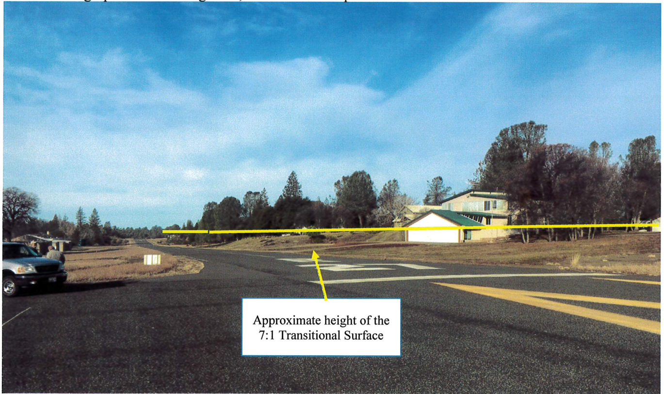
Photograph 12 – Looking east, trees and brush penetrate the 7:1 Transitional Surface.
