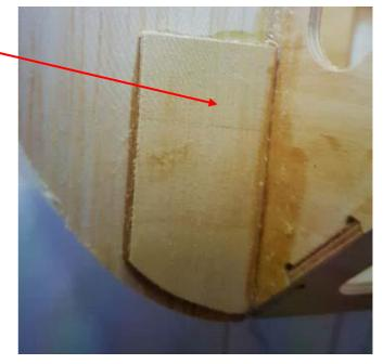
Position the lower cowl rings against the spacer / F2. Make sure to align the cowl ring slightly inset from the fuselage sides to account for the thickness of the cowl.
