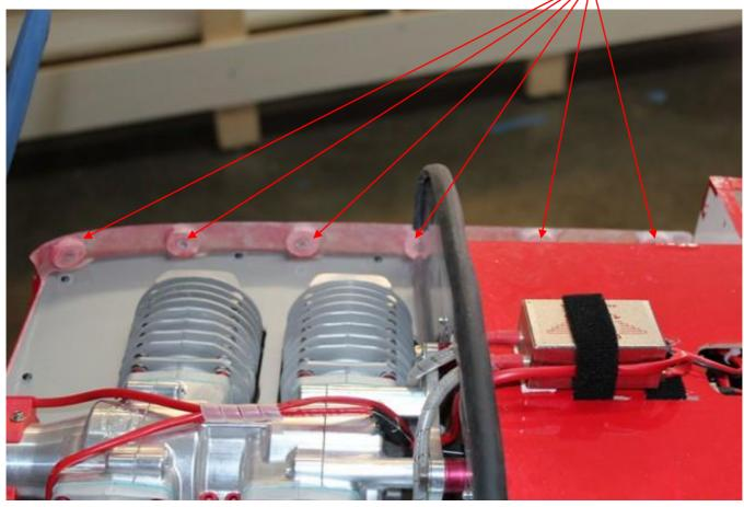
Install the anchor pads (with blind nuts installed) to the lower half of the cowl with epoxy. I complete this step with the cowl halves still mounted to the airframe and taped together by using a bolt at each pad location to pull it snug to the cowl. Note: Do not tighten the bolt so much that you squeeze all the glue out of the joint.
