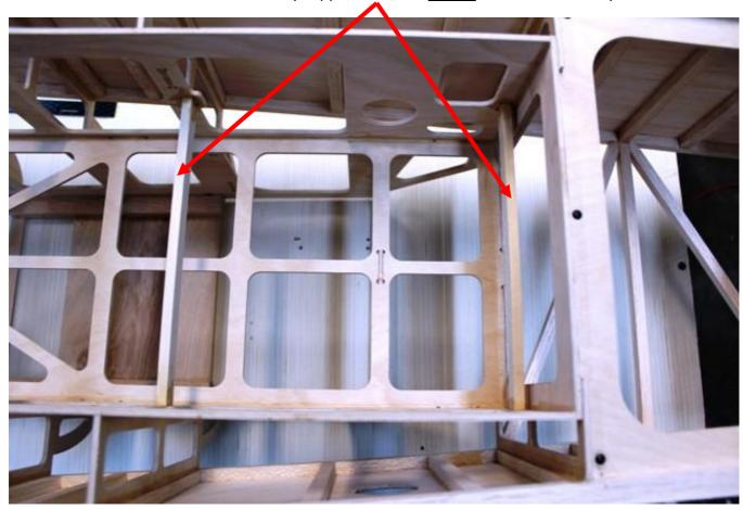
This completes the motor box assembly, and it is now ready to be mated to the fuse sides. The next chapter will detail the construction of the fuselage sides.
