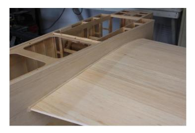
Note: When trail fitting the wings, make sure they aligned at or very close to the proper incidence setting.
