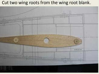
Locate the 48" x 3/8" x 4" wing root blank.
