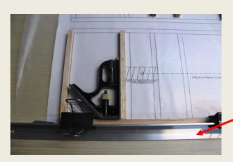
1" x 1" x 96" Aluminum angle stock. - With the longeron clamped in place, locate and glue in place the upper longeron plate support rail. Note: make certain it is oriented in the proper direction.
