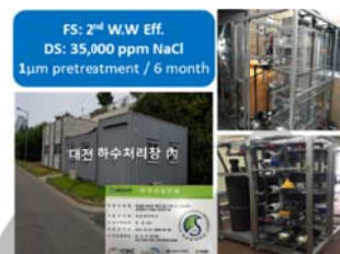
Figure 1. Element scale plate-frame FO (PFFO) system operated at real site
