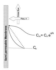
One EIS-derived parameter is the normalized conductance of the diffusion polarization ( $G_{DP}$ ) layer which is located within the concentration polarization layer.
