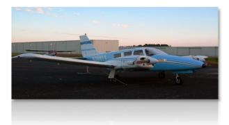
The **Piper Seneca** (PA-34-200) is a six seat, twin engine, low wing airplane. The engines are 200 horsepower each. The **Seneca** adds power and performance while still retaining the safety of counter-rotating propellers.
