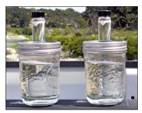
The effluent sample on the left, discharged from an Orenco AX100 Treatment System, is as clear as the water sample on the right, taken from a nearby lake.
