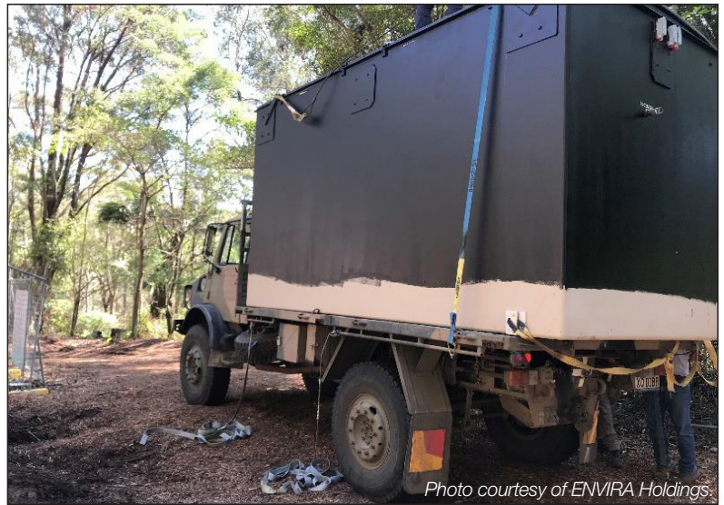
The versatility of the AX-Max design allowed it to be split into two units per site, so that each unit could be transported up the mountain via truck. To blend in more fully with the environment, each unit received a custom paint job.
