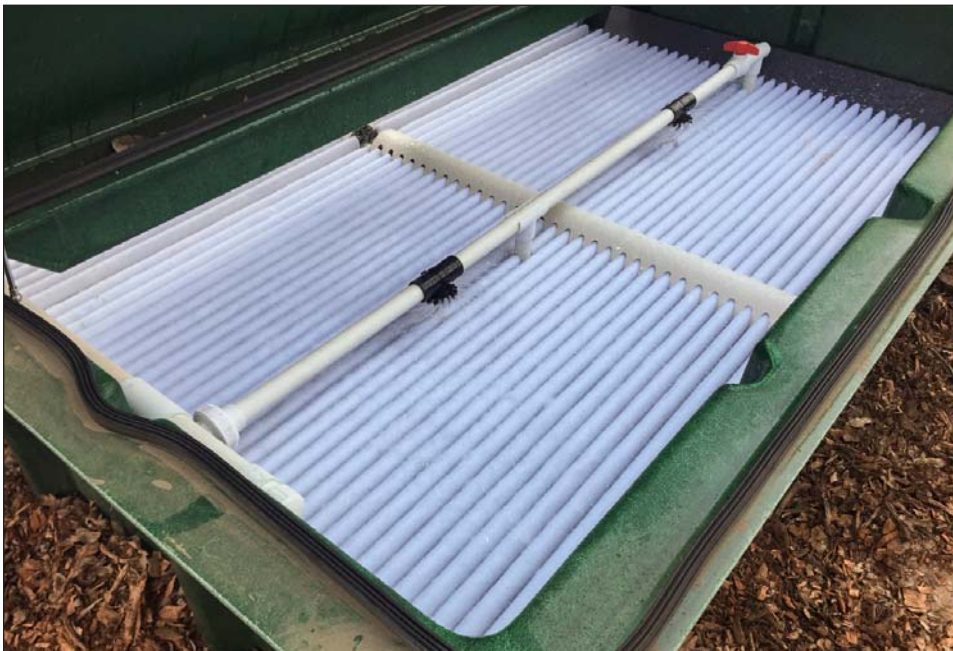
Treatment media in the AdvanTex AX100 is a uniform, engineered textile, which is readily serviceable and allows significantly higher loading rates than traditional recirculating gravel or sand filters.
