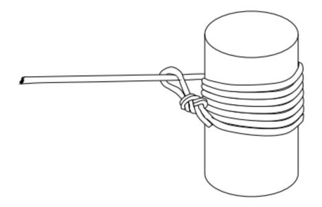
Tie a "figure 8 on a bight" or a "bowline" on the working end of the rope, and connect this knot to the standing rope just in front of the first wrap by using a steel carabiner. It is also acceptable to simply tie the tail of the last wrap around the standing part of the rope.
