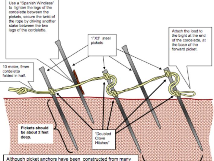
Although picket anchors have been constructed from many types of material, the material of choice is "T" shaped steel stakes, a least three feet long. These stakes are commonly used for range fences. Rolled steel stakes, used to secure concrete forms, are also used for picket anchors. "T" stakes work better in loose soil or sand, preventing the "plowing" of the ground, while rolled steel may be better suited for hard rocky ground because of better penetrating qualities.
