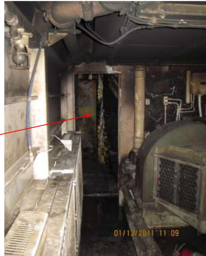
Operate the foam line from this door into the engine compartment.
