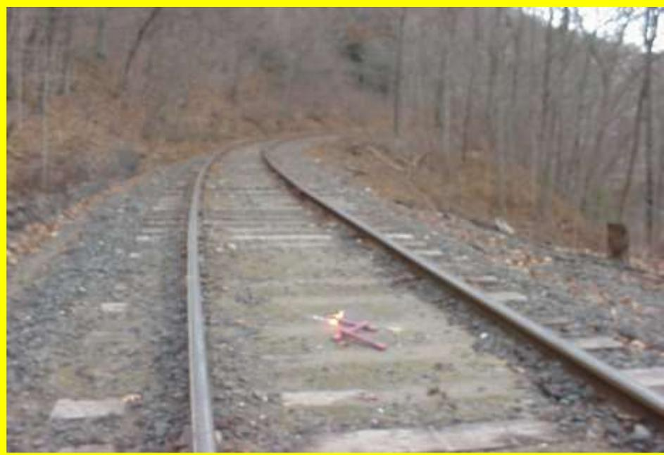
Place a lighted flare between the rails, on ballast, out about 2 miles in both directions from the incident location.
