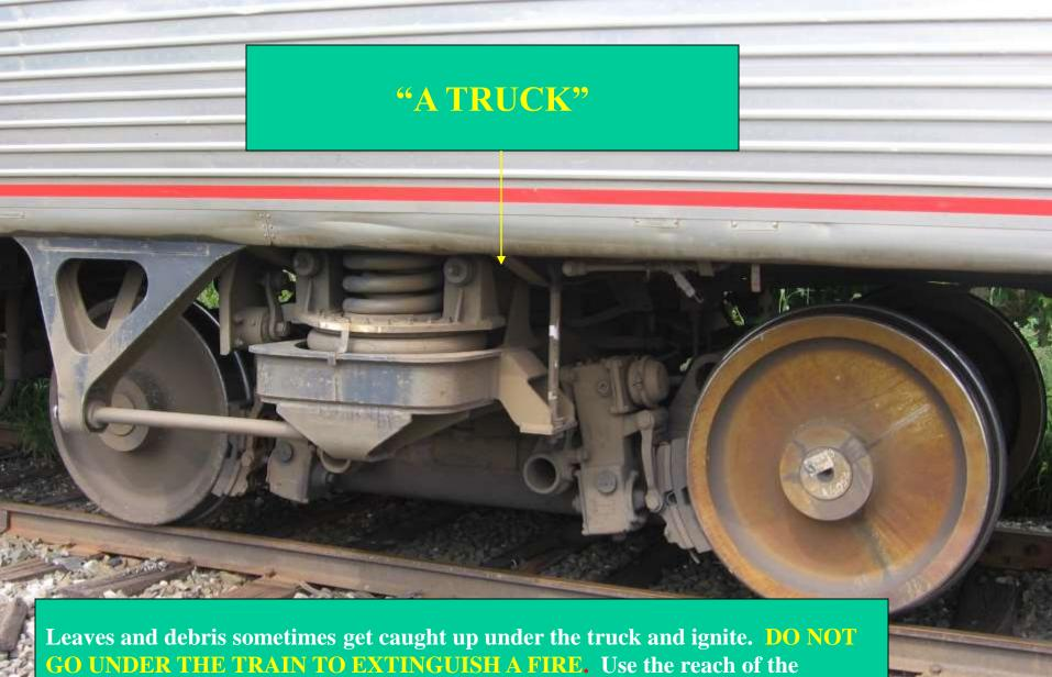
stream of an ABC multi-purpose dry chemical extinguisher to extinguish a fire in this area.
