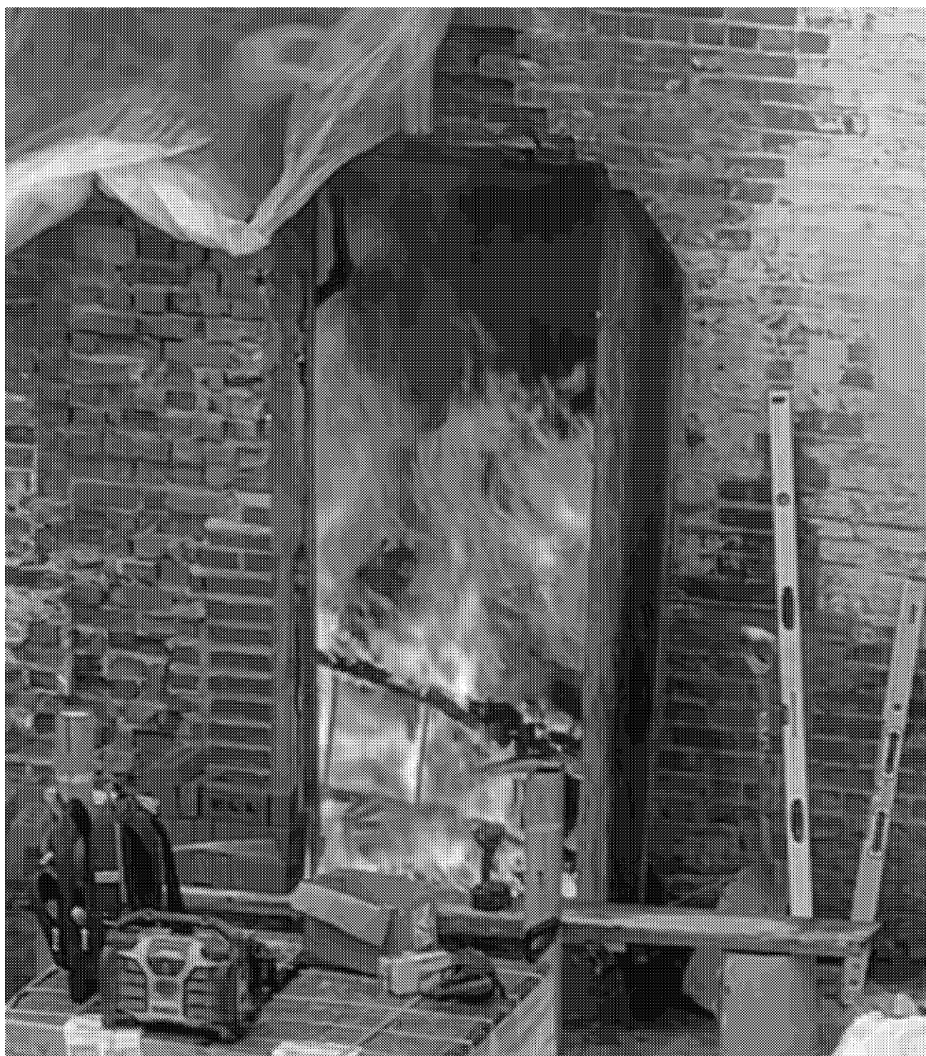
Figure 24 - Charring on the east interior face of the plywood
