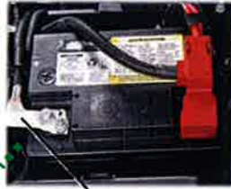
Cut here to disable BOTH 12v negative cables at once
