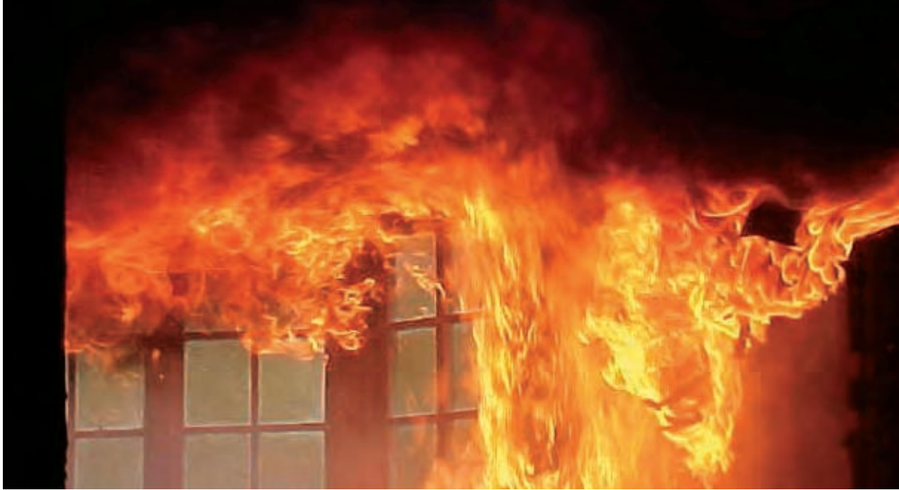
Figure 29. The fire is starting to approach flashover and the radiation to all the other parts of the fire room is increasing.
