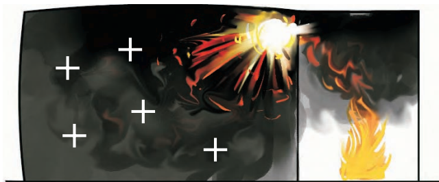
Figure 114. The smoke gases have leaked into the adjacent room and are ignited by a shooting flame.
