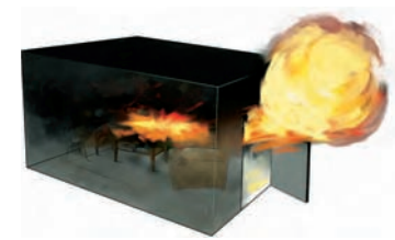
Figure 92. Premixed area ignites, which corresponds to the dark area.
