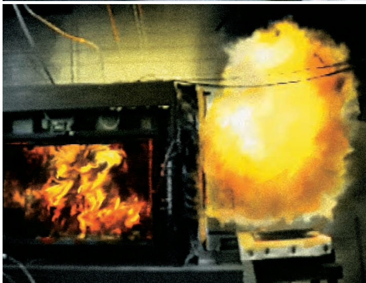
Figures 99 and 100. The fire ball formed due to the expansion of the smoke gases.
