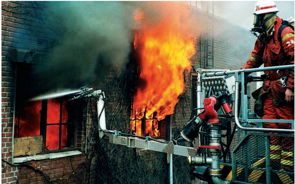
Figure 110. The fixed lance version of the cutting fire extinguisher.
