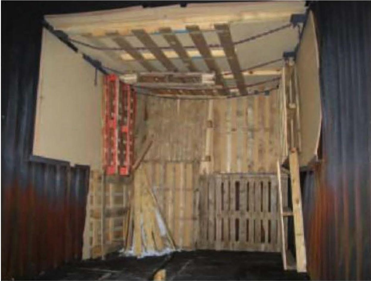
*Photograph No 6 – Fire Development Simulator (FDS) pre-loaded with 2.44m x 1.22m x 12.5mm soft board sheets used as wall and ceiling linings*
