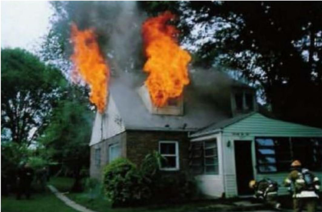
*Photograph No.12. – Flames issuing from the bottom of the window sill upwards from an upper floor window*
