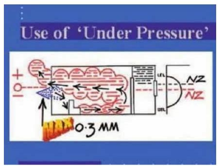
Figure No.18 – Use of the 'under pressure' extinguishing technique
