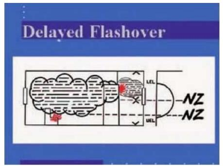
Figure No. 22 – Open Ignition Source for a 'Delayed Flashover' in the corridor
