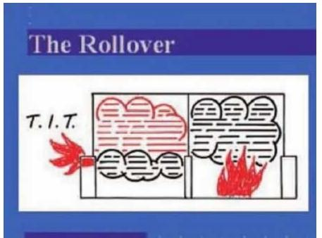
Figure No.36 – 'The Rollover' exits the building into the street
