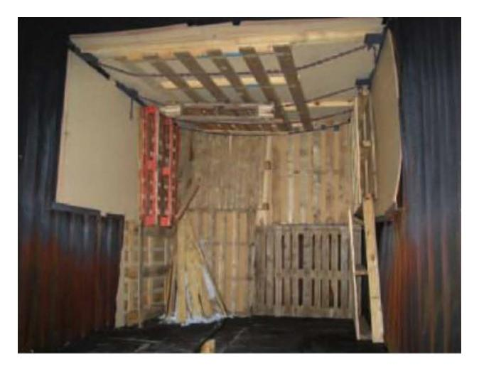
Photograph No 6 – Fire Development Simulator (FDS) pre-loaded with 2.44m x 1.22m x 12.5mm soft board sheets used as wall and ceiling linings
