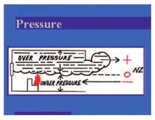
Figure No. 1 – Over Pressure, Under Pressure and Neutral Zone (NZ)
