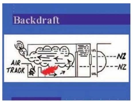
*Figure No.12- Backdraft (Ventilation Induced Flashover)* The second type of flashover is called a '**backdraft'.**
