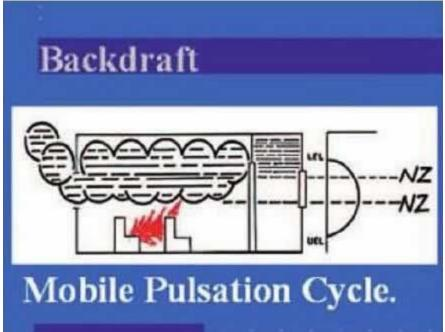
Figure No. 15 – 'Backdraft' – Mobile Pulsation Cycle (Positive Mode)
