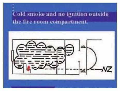
Figure No.31 – Cold smoke and no ignition outside the fire room compartment
