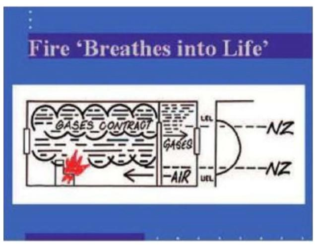
Figure No. 9 The fire 'breathes into life' stage
