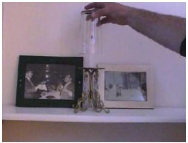
Photograph No.8.d. – Flame extinguished inside glass placed half over a candle
