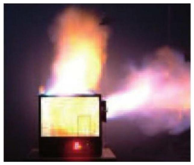
Photograph No. 4 – A 'fire gas explosion'
