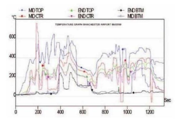
Figure No.30 – Temperature monitoring chart from inside the Fire Development Simulator (FDS)
