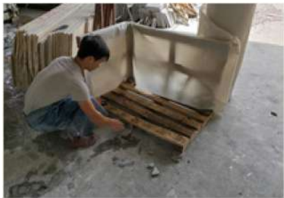
1. Putting the foam into the base of wooden case
