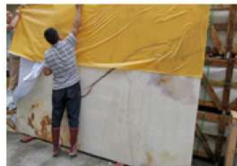
1. Covering the slabs by masking tap
