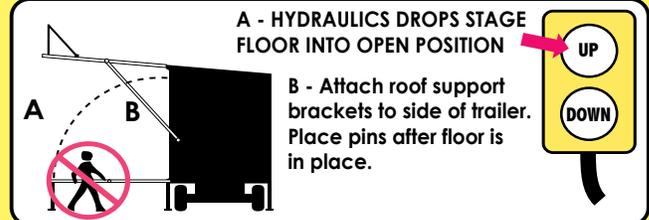
A - HYDRAULICS DROPS STAGE FLOOR INTO OPEN POSITION
