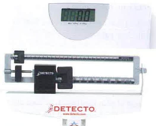
Fig. 14-24. The scale must be balanced at zero before beginning to obtain a client's weight. On the top is a digital scale and on the bottom is a standing scale. (PHOTO COURTESY OF DETECTO, WWW.DETECTO.COM, 800-641-2008)
