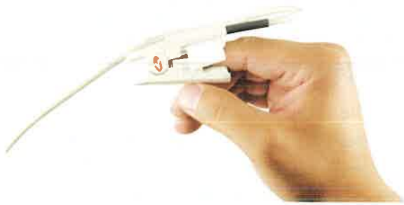
Fig. 14-16. A pulse oximeter sensor is usually clipped on a person's finger to measure the amount of oxygen in the blood, as well as pulse rate.
