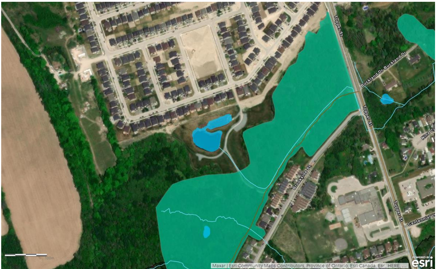
A two-stage water quality and water quantity stormwater ponds at the centre of the map, located at the new Towerhill Highlands community in Millbrook. Wetlands adjacent the ponds provide habitat and groundwater discharge. Connecting streams and ditches connect the ponds with the natural system and into Baxter Creek. Map courtesy: Baxter Creek Watershed Hub, Baxter Creek Watershed Alliance.
