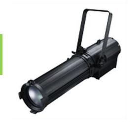
Solar Pro 200Za CC is ERS-style fixture with manual zoom range of 12° - 30°. It is constructed using high-precision HD optics encased in rugged housings designed to survive the rigors of touring, broadcast and theatrical production. Control options like selectable PWM, RDM, and selectable dimming curves round out this virtually silent ellipsoidal.
