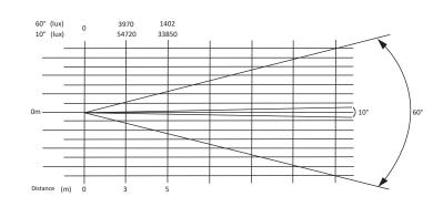
The BEE EYE K15 is a powerful LED moving head wash with 19pcs 25W RGBW Prolight LEDs, offering a versatile beam angle of 10° to 60°. It features individual LED control, a color temperature range of 2500K-8000K, and dynamic effects like "vortex" and "kaleidoscope." With 4 linear dimming curves and strobe effects from 1-25 Hz, it provides professional-grade performance for any event.
