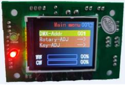
Operational instructions: Under the main menu, press the up and down keys to select different function menus, select different function menus, then press the confirmation key to enter the corresponding pull-down menu functions, and press the increase or decrease key in the pull-down menu to modify its parameter values. Press the confirmation key to return to the main menu.
