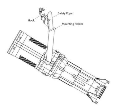
Please use qualified safety-rope, which can hold at least 10 times the weight of the fixture. You must only use safety-ropes with quick links with screw cap. Pull the safety-rope through the hole on the bottom of the base and over the trussing system etc. Insert the end in the quick link and tighten the fixation screw. A safety rope which already hold the strain of a crash or which is defective must not be used again.
