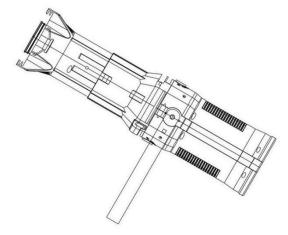
■ When rigging the devices on the truss and the head face to the floor. Screw one clamp each via a M12 screw and nut onto the mounting holder. Insert the quick-lock fasteners of the first mounting holder into the respective holes on the bottom of the device. Tighten the quick-lock fasteners fully clockwise. Install the second mounting holder. And the safety rope must be used at same time.
