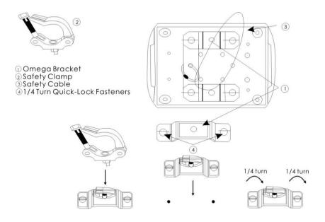
Regardless of the rigging option you choose for your LED moving head, always be sure to secure your fixture with a safety cable. The fixture providers a built-in rigging point for a safety cable on the hanging bracket as illustrated above. Be sure to only use the designated rigging point for the safety cable and never secure a safety cable to a carrying handle.
