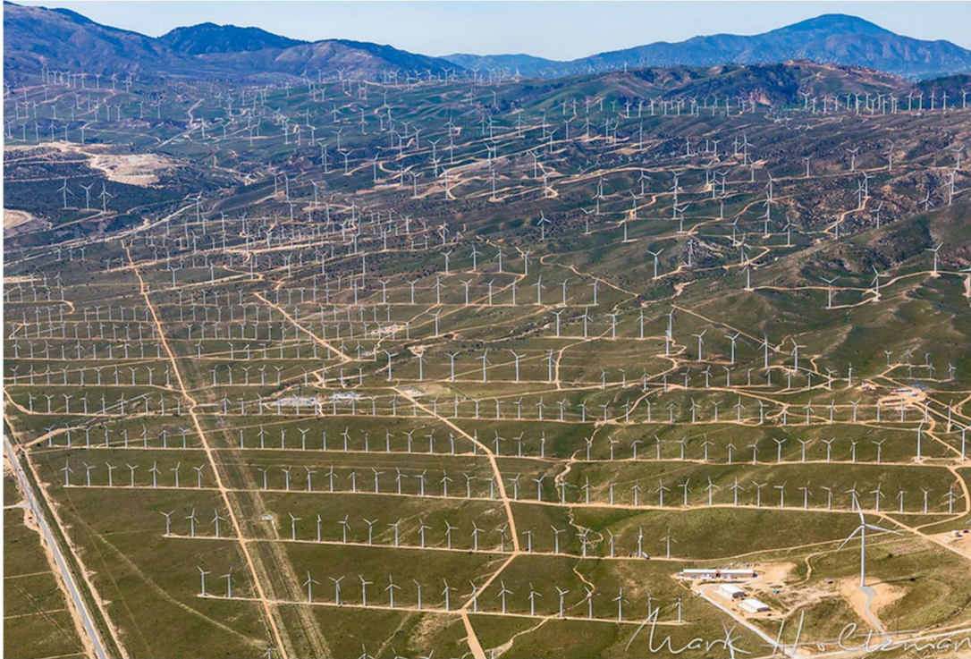
Alta Wind Energy Center, Kern County California: : 830 MW electricity generation. Project land requirements: 3,200 acres. Project Cost: $2.87 billion. Produces “clean energy” for up to 257,000 homes.
